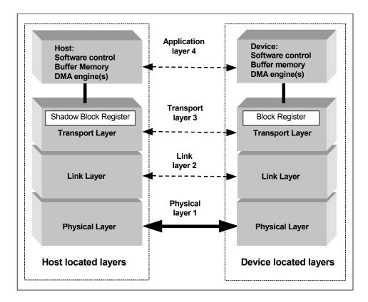
Figure 5.3 Conceptual diagram of communication layers
